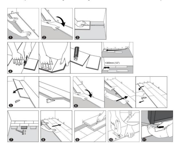
1. **First row, first plank:** After thoroughly cleaning the subfloor, you should begin laying from left to right. Position the first plank so that the grooved edge is facing you. Place the floorboard 1/4" / 6 mm from the left wall. Use spacers between the wall and the floorboard.
