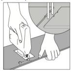
11. **Door molding and skirting:** Lay a tile (with the decorative side down) next to the door molding and saw as shown in the figure. Then slide the floorboard under molding.
