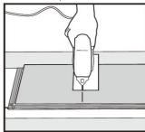
3. **First row, first tile:** After adjusting, the measurements of the first tile as described above, begin laying at the left-hand corner of the longest wall and proceed from the wall with the tongue sides facing walls and the grooves facing outward, away from the walls. Use spacers between the wall and the tile to create ½" / 10 mm expansion gap and to keep a straight line parallel to the abutting wall.
