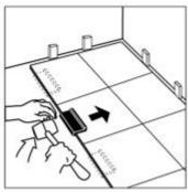
**Tip:** After the first 2-3 rows of tiles are installed, they should be checked with a string line to ensure that rows are still running straight. If they are not, it could be that the starting wall has some irregularities that caused bowing in the installation. If so, the starting row of tiles may have to be scribed and re-trimmed to account for any unevenness in the wall. This can be done without having to disassemble the beginning rows.
