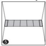
6. **Second row, first tile:** Click the tongue side of the tile into the previous row with both groove sides facing out at an angle of 25-30°, slide towards the wall (respect the ½" / 10 mm expansion gap) and fold down, ensuring that the long side is fully engaged with no visible gaps, and that the right edge of the tile is perfectly aligned with the first tile of the first row.
