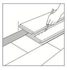
10. **Holes for pipes:** Measure the diameter of the pipe and drill a hole that is 7/8" / 20 mm larger. Saw off a piece as shown in the figure and lay the board in place on the floor. Then lay the sawed-off piece in place.
