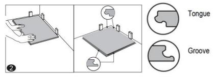
4. **First row, second tile:** Lay down the second tile on the right-hand side of the first tile, aligning its left side over the right-side groove of the first. Make sure both tiles are perfectly aligned. Gently tap down with a rubber mallet to lock it into the groove of the first tile, until both are at the same height. The mallet should hit the tile directly above the locking system, allowing for a correct engagement.
