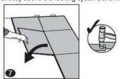
8. **After finishing the installation of every row:** Use a tapping block or cutoff and a rubber mallet to gently tap the tiles into the click of the previous row to make sure they are tightly clicked together and make sure there is no gap between the long sides of the tiles installed. Any gapping can compromise the whole installation.
