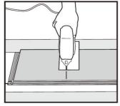
3. First row, first tile: After adjusting the measurements of the first panel as described above, begin laying at the left-hand corner of the longest wall and proceed from the wall with the tongue sides facing walls and the grooves facing outward, away from the walls. Use spacers to create ½" / 10 mm expansion gaps.
