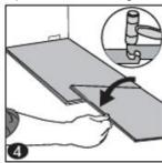
5. First row, last tile: At the end of the first row, leave an expansion gap of ½" / 10 mm to the wall and measure the length of the last tile to fit.
