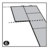
7. **Second row, second tile:** Lay down the second tile on the right-hand side of the first tile by clicking it into the previous row at a 25-30° angle, aligning its left side over the right-side groove of the first. Make sure both tiles are perfectly aligned. Gently tap down with a rubber mallet to lock it into the groove of the first tile, until both are at the same height. The mallet should hit the tile directly above the locking system, allowing for a correct engagement.
