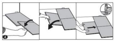
5. **First row, last tile:** At the end of the first row, leave an expansion gap of ½" / 10 mm to the wall and measure the length of the last tile to fit.
